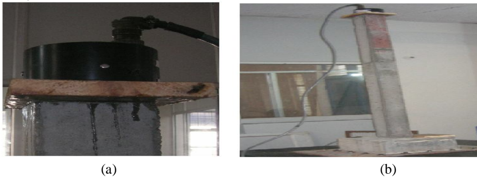
FIGURE 2.1 Experimental set - up (a) Schematic view RC column model in the laboratory (b) Location of the sensor placed at top of the RC column
